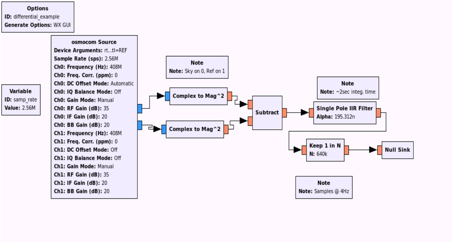
In the so-called *flow-graph* shown above, the two complex base-band data streams are delivered to a block that acts like a conventional detector, computing:
