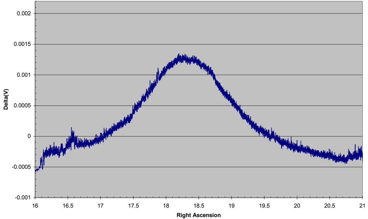
Below, we show the plot of a daily solar transit, recorded at both 10.7cm and 2.6cm wavelengths, where the 10.7cm data are derived from a *fixed-load* differential radiometer, and the 2.6cm, from a *reference-beam* differential radiometer, as described previously.
