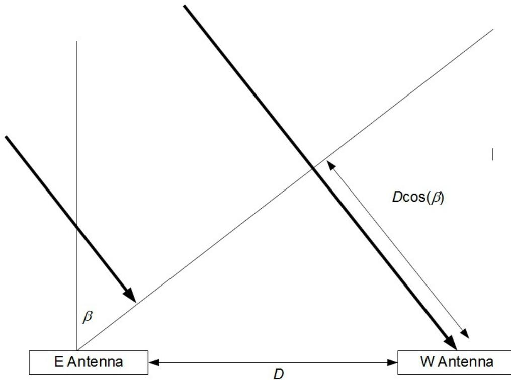
Two antennas, separated by a distance  $D$  are observing a source at an angle  $\beta$  from the meridian. The signal reaching the west antenna has an additional distance of  $D\cos(\beta)$  to travel. This corresponds to a phase difference of:
