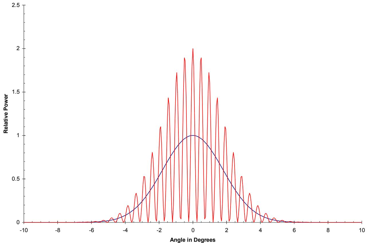
The black line shows the sensitivity pattern of the individual antennas; the red line shows the interference pattern due to the interferometer. The hardware arrangement is shown below.
