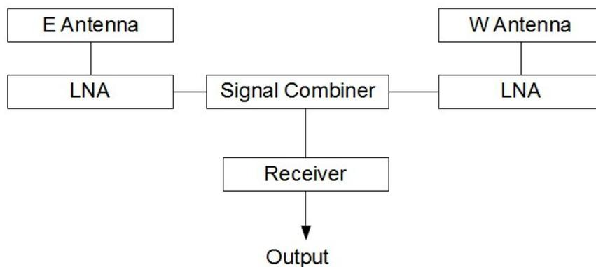
Low noise amplifiers are included at the antennas because of the losses due to the long cable lengths running along the interferometer baseline. We assume here the lengths are equal, although they don't really have to be.
