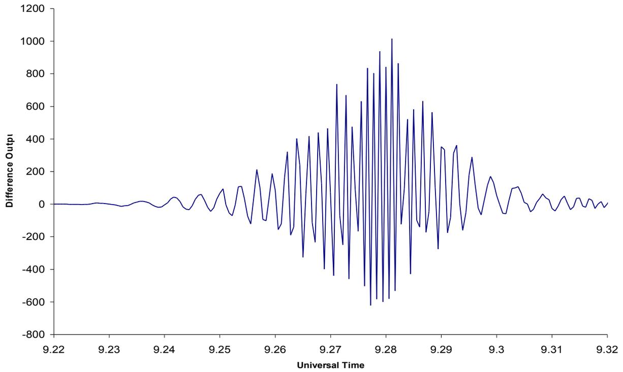
In both cases the transits show some asymmetry, probably due to a combination of the phase shift not being exactly 180 degrees (a half-wavelength piece of coax was used) and also the gain of both LNA+receiver channels probably differ slightly.
