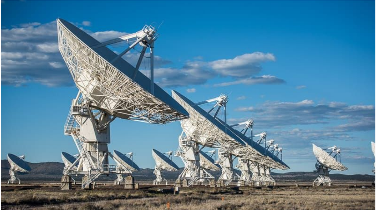
Fig. 3: The Very Large Array (VLA) is one of the most sophisticated radio telescope arrays in the world, consisting of twenty-seven 25-meter radio antennas that can function as a high-resolution radio interferometer.
