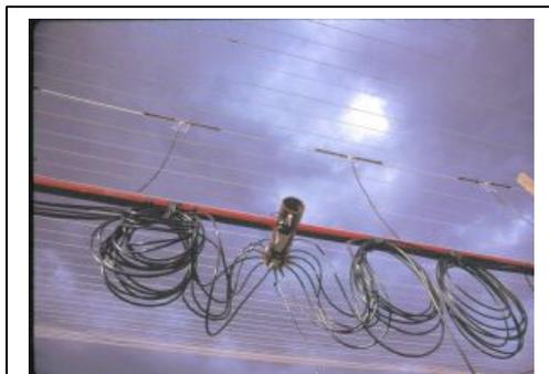
**FIG. 5-**"Medusa", one of the two 12-way signal combiners. These are quarter-wave sections of coaxial line which match 12 50-ohm lines in parallel (an impedance of 4 ohms) to the 50-ohm cable transferring the combined signals to the GaAsFET amplifiers. They are constructed from copper tube and have an effective bandwidth of at least 10 MHz
