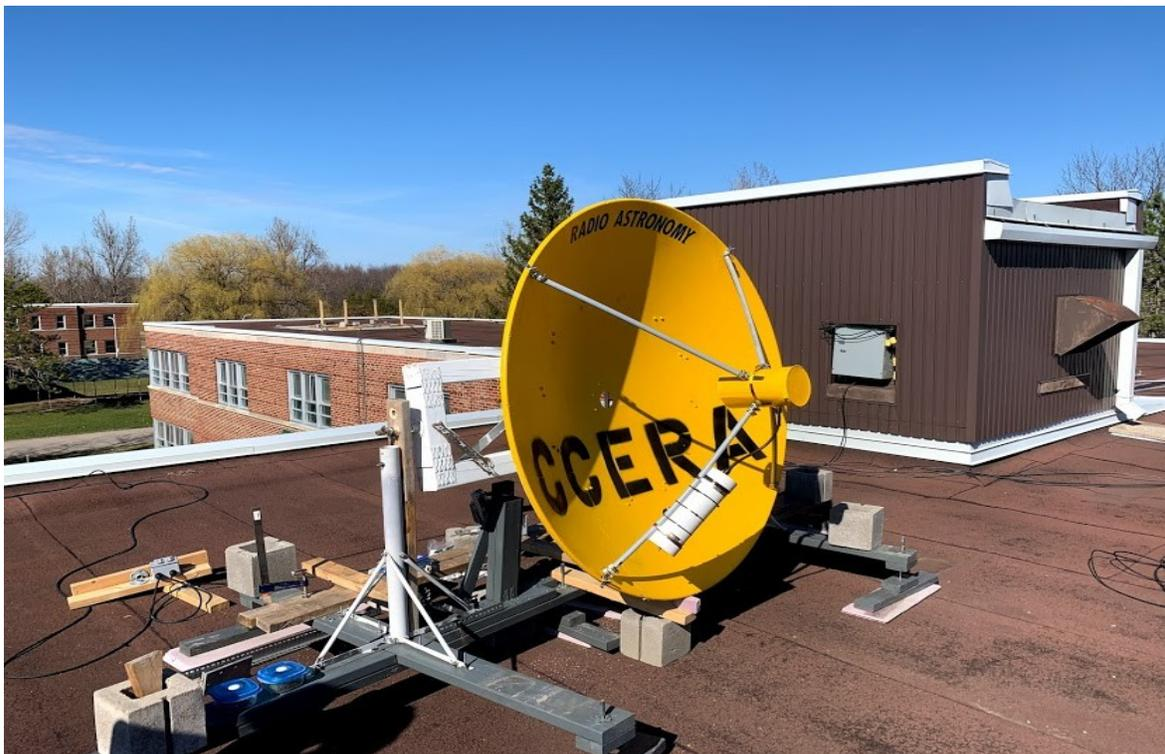
The feed is connected to an off-the shelf Low Noise Amplifier (LNA) assembly, providing approximately 40dB of sub-0.7dB NF gain. The LNA was provided by *NooElec*<sup>1</sup> as a prototype
