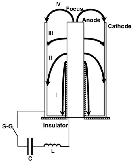
**Figure 1.** A scheme of the equivalent circuit and the plasma dynamics are shown. The capacitor C is discharged over the electrode through a spark gap (SG). The plasma dynamics is sketched in a side section of the electrodes, I: the discharge starts over the insulator, II, III: the current sheath is accelerated along the coaxial electrodes and IV: pinch.
