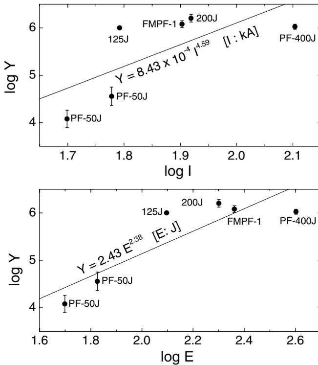
**Figure 2.** Neutron yield,  $Y$ , scaling laws for sub-kilojoules PF devices ( $I$ : current,  $E$ : stored energy). Data include results from CCHEN (PF-400J [6], PF-50J [8]) and others groups (125 J [10], 200 J [11], FMPF-1 [12]).
