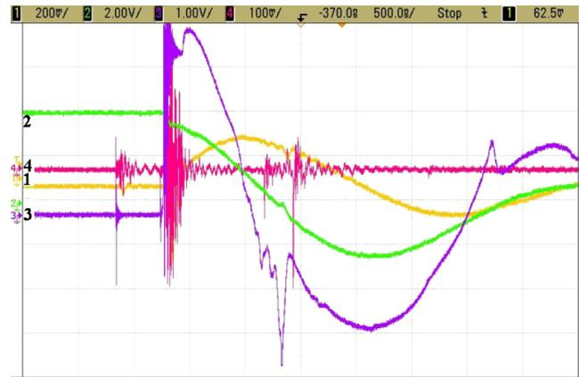
FIG. 5. (Color online) Double pinch in  $D_2$  plasma focus. 1: current (5 mV/kA). 2: voltage (1 V/kV). 3:  $di/dt$ . 4: PMT output; horizontal axis 500 ns/div.
