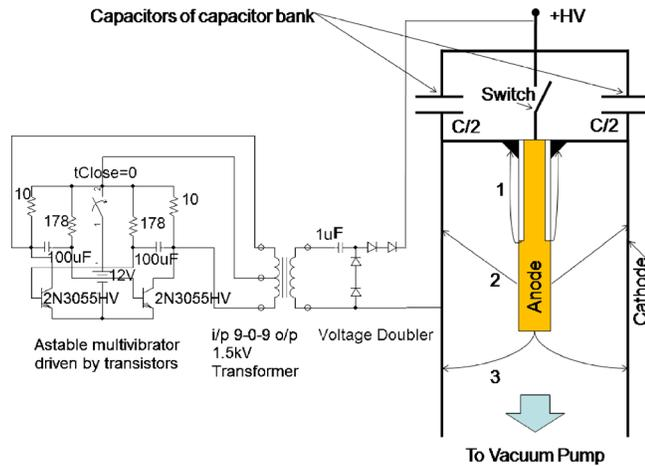
FIG. 1. (Color online) Schematic of Mather type plasma focus. 1: breakdown phase. 2: axial acceleration phase. 3: radial compression phase.
