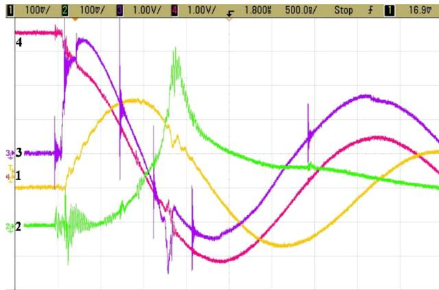
FIG. 4. (Color online)  $H_2$  plasma focus. 1: current (5 mV/kA). 2: photodiode output. 3:  $di/dt$ . 4: voltage (1 V/kV); horizontal axis 500 ns/div.
