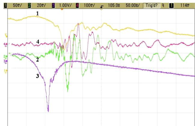
FIG. 6. (Color online) Time-of flight signal of neutron and hard x-ray in  $D_2$  plasma focus. 1: current (5 mV/kA). 2: PMT1 output. 3:  $di/dt$ . 4: PMT2 output; horizontal axis 50 ns/div.
