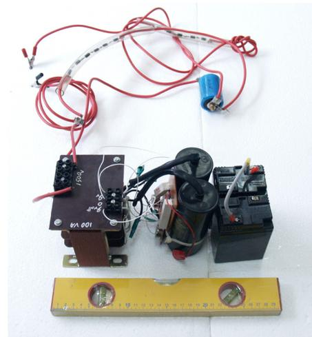
FIG. 3. (Color online) Battery driven compact power supply for plasma focus.
