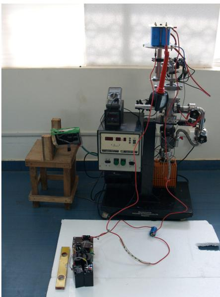
FIG. 2. (Color online) Experimental setup of plasma focus.
