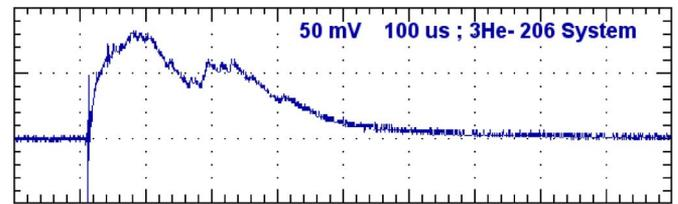
Fig. 4. Electrical signal delivered by one of the  $^3\text{He}$ -filled proportional counters. The spread in the timescale and the piled-up electrical signals of the neutrons are determined by the moderator effect as it is explained in [6].
