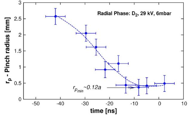
Fig. 3. Radial phase dynamics from interferometric measurements. Zero time referred to time of dip occurrence in  $dI/dt$  signal. Pinch formation close to zero time.
