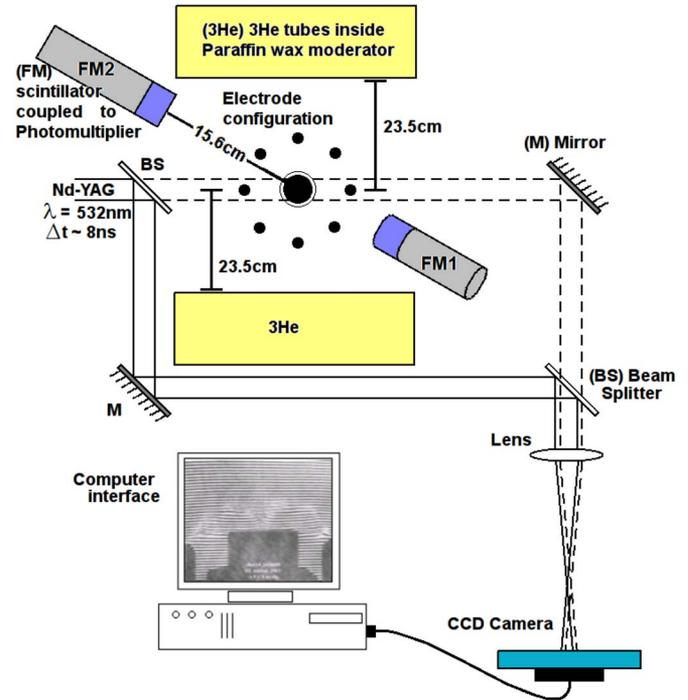
Fig. 1. Schematic diagram of the experimental setup. Electrode configuration is shown at the middle of the two  $^3\text{He}$  detectors.
