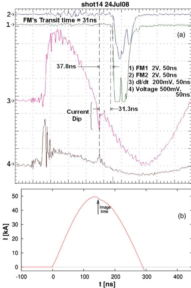
Fig. 5. (a) Electrical and scintillator assembly signal. Assemblies FM1 and FM2 were placed at 15.6 cm from anode axis. The transit time of 31 ns in the photomultiplier tubes must be considered. (b) Current signal from numerical integrated  $dI/dt$  signal. Time referred to start of  $dI/dt$  signal.
