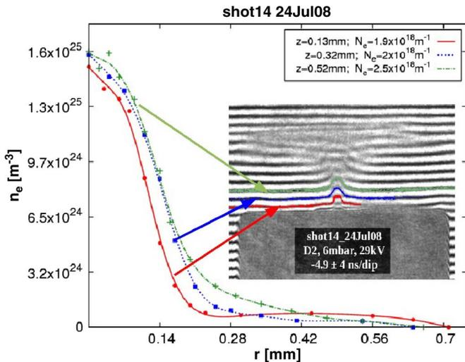
Fig. 6. Electron density profiles obtained by Abel inversion of fringe shifts from interferograms for shot14\_24Jul08.
