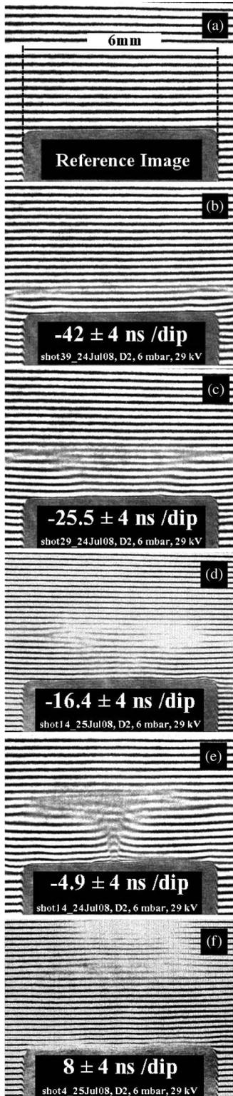
Fig. 2. Interferometric sequence for the radial and pinch phases. (a) Spatial reference image. (b) Early radial phase. (c) and (d) Radial phases close to time of maximal radial piston velocity, around  $10 \text{ cm}/\mu\text{s}$ . (e) Pinch phase (note the formation of a high-density column). (f) Time after column disruption (note remaining material over the place of previous column formation).
