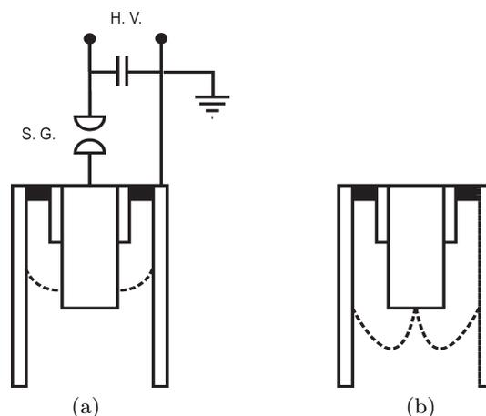
**Fig. 1.** Schematic of plasma sheet: (a) in the coaxial stage and (b) radial compression stage.
