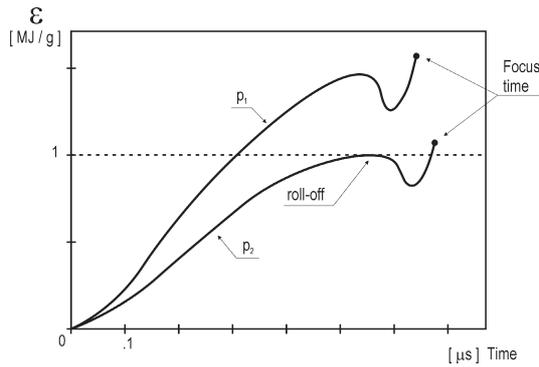
**Fig. 2.** Typical curves of the electromechanical work performed on a deuterium plasma focus sheath by mass unit  $\varepsilon$  as a function of time for two different values of the pressure  $p_1$  and  $p_2$ . The horizontal dotted line indicates the specific ionisation energy of deuterium.
