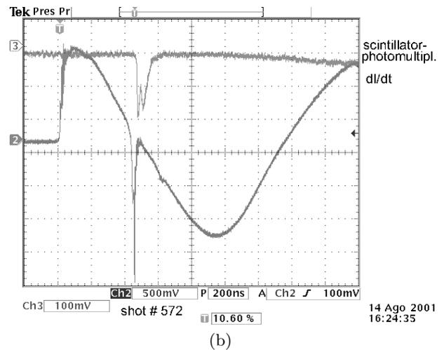
**Fig. 7.** Two typical oscillograms obtained in discharges of Nanofocus. The respective lower traces correspond to Rogowski's current derivative signals. The upper traces show the signals coming from the scintillator-photomultiplier detector.
