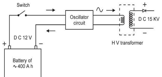
**Fig. 4.** Scheme of a portable power supply for the capacitor charge, based in a tractor battery.
