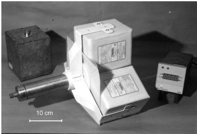
**Fig. 5.** General view of the Nanofocus with the capacitor bank in “star” disposition.
