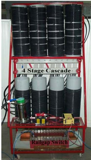
**Figure 4.** Experimental layout of the Cascaded Pulser
