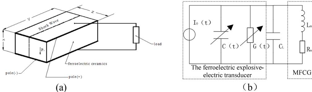
Fig.2 The schematic diagram of the ferroelectric explosive-electric transducer and its equivalent circuit
