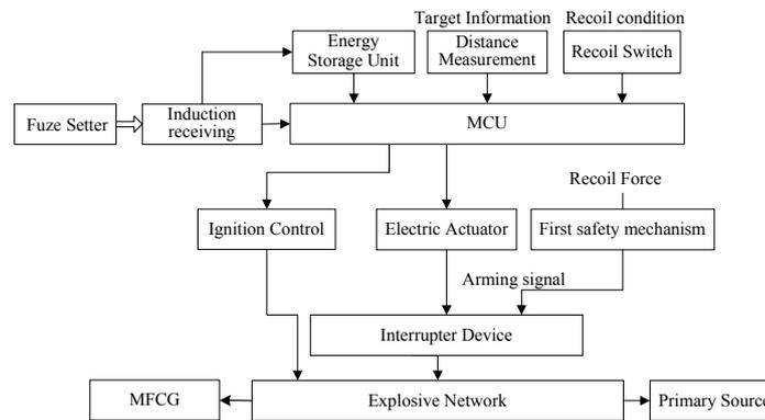
Fig.6 Principle block diagram of safety and arming system
