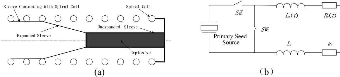
Fig.3 Action process of MFCG and its equivalent circuit
