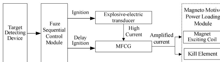
Fig.1 Principle block diagram of MAHEM
