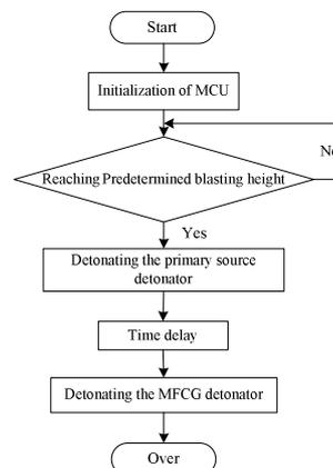
Fig.5 The flow chart of detonating time sequence
