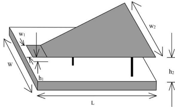
**Figure 5.** Geometry of the Half TEM Horn Antenna
