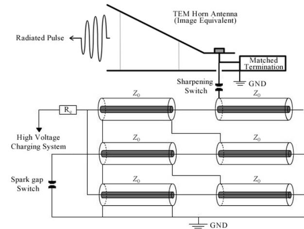
Figure 1. Schematic layout of EMI Generator
