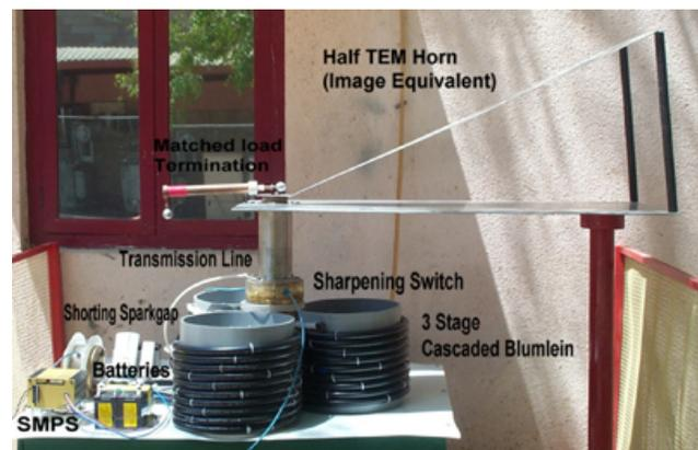
**Figure 6.** Experimental layout of the RF Source system
