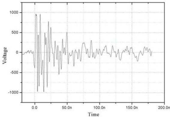
**Figure 3.** Radiated Impulse from Half TEM Horn
