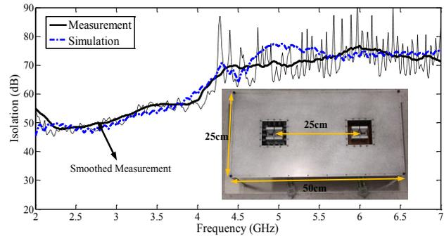
Fig. 4. Measured and simulated isolation of the proposed bistatic STAR system.
