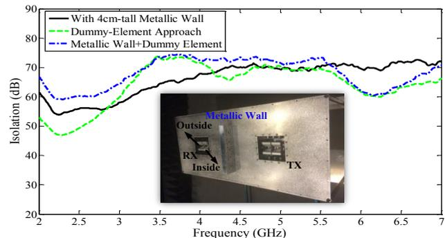
Fig. 5. Measured isolation of the proposed bistatic system with a metallic wall inserted as shown in the inset and with the dummy-element approach.
