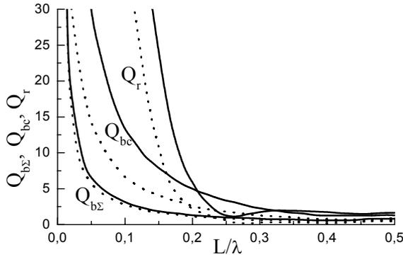
Fig. 2. Partial Q-factors of  $2L$  length dipole versus  $L/\lambda$ .
