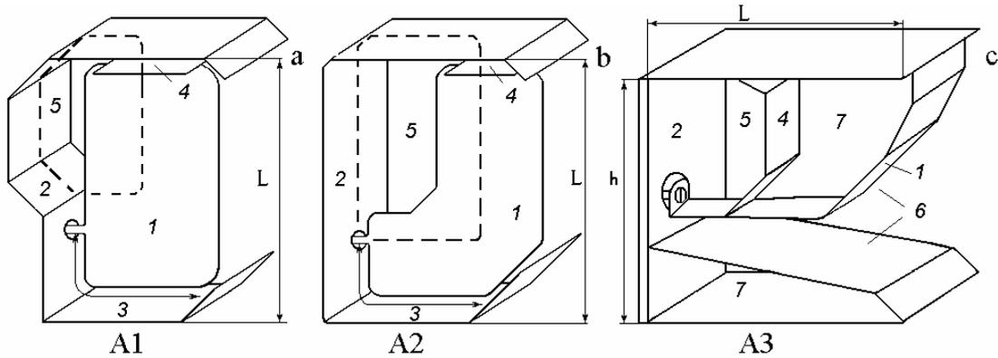
Fig. 4. Combined antennas geometry. 1 – electrical monopole, 2 – case, 3 – slot line, 4 – plate, 5 – active magnetic dipole, 6 – TEM-horn, 7 – passive magnetic dipole.
