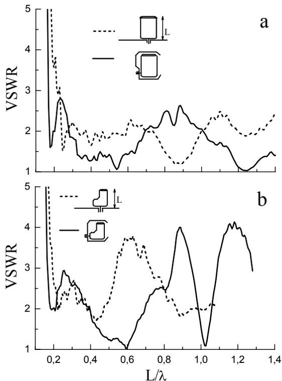
Fig. 5. VSWR of electrical monopole and A13 antenna (a), monopole and A22 antenna (b).
