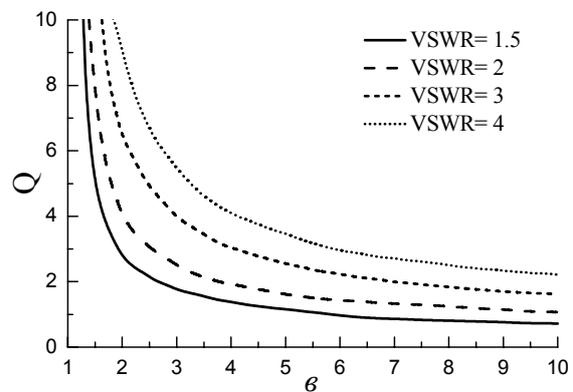
Fig. 1. Q-factor versus frequency overlapping for different VSWR.
