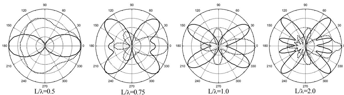
Fig. 3. Electrical dipole patterns:  $2\theta_0 = 180^\circ$  (solid lines),  $2\theta_0 = 90^\circ$  (dash lines).
