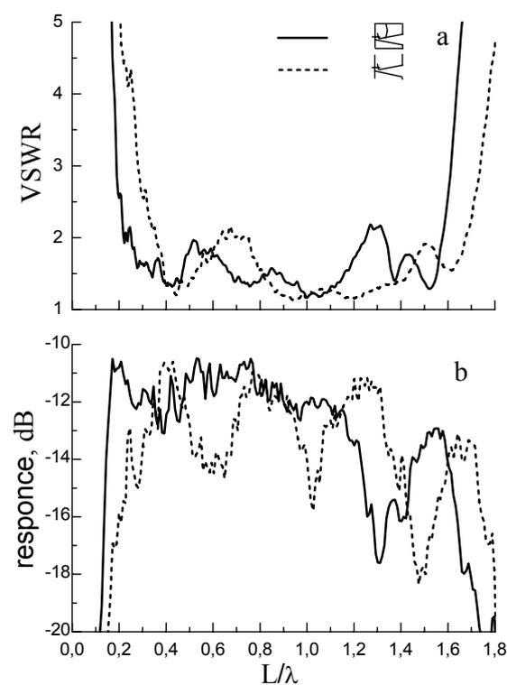
Fig. 6. VSWR (a) and amplitude frequency response (b) of TEM-horn and A32 antenna.
