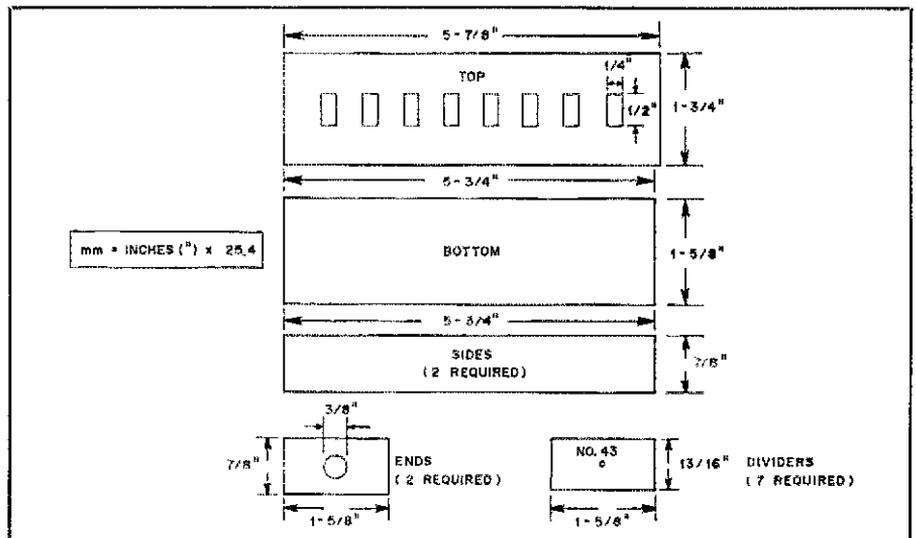
Fig. 2 — Mechanical dimensions of the attenuator enclosure.
