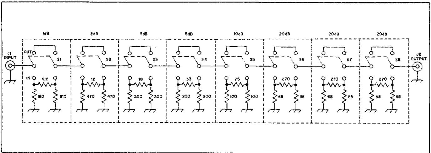
Fig. 1 — Schematic diagram of the attenuator. Resistors are 1/4-W, 5%-tolerance, carbon-composition or film types. Resistances are given in ohms.
